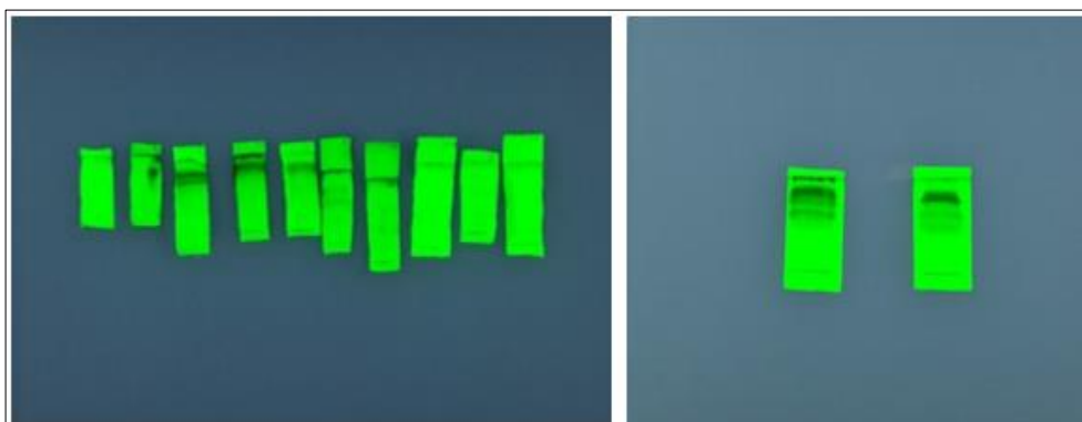
Plate 1: TLC plates of samples visualized under 254 nm of (A) column eluted fraction & (B) crude methanolic extract of Adulsa in same solvent system
